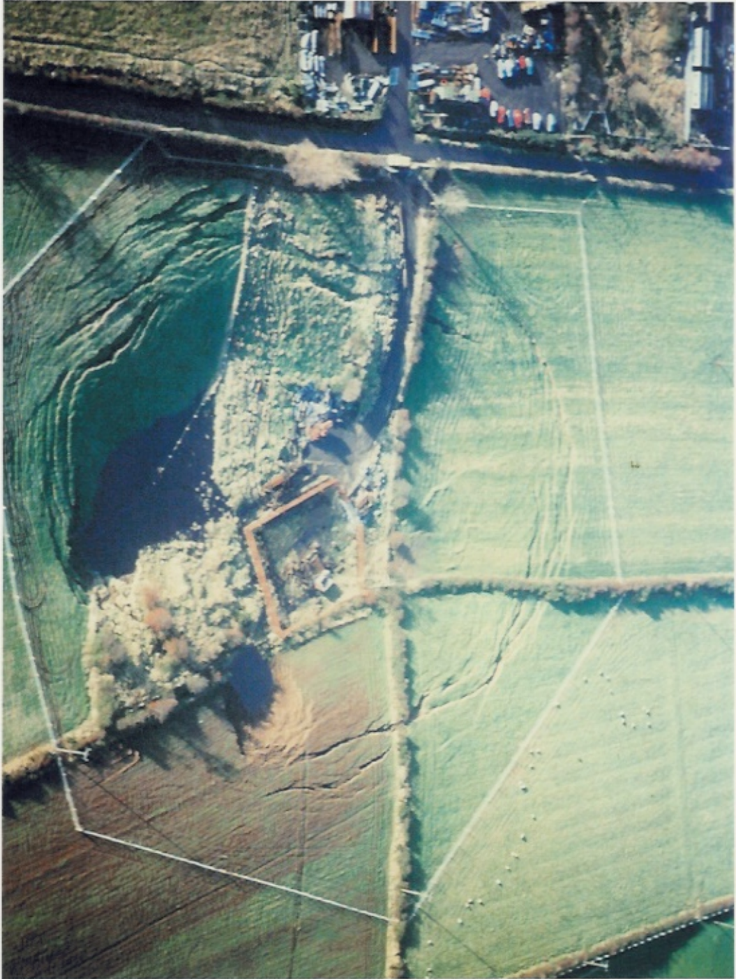
The collapse of a disused salt mine at Carrickfergus, Co. Antrim on 19 October 1990 had the seismic effect of a magnitude 2.5 earthquake. (Photograph: BGS Belfast Office)
