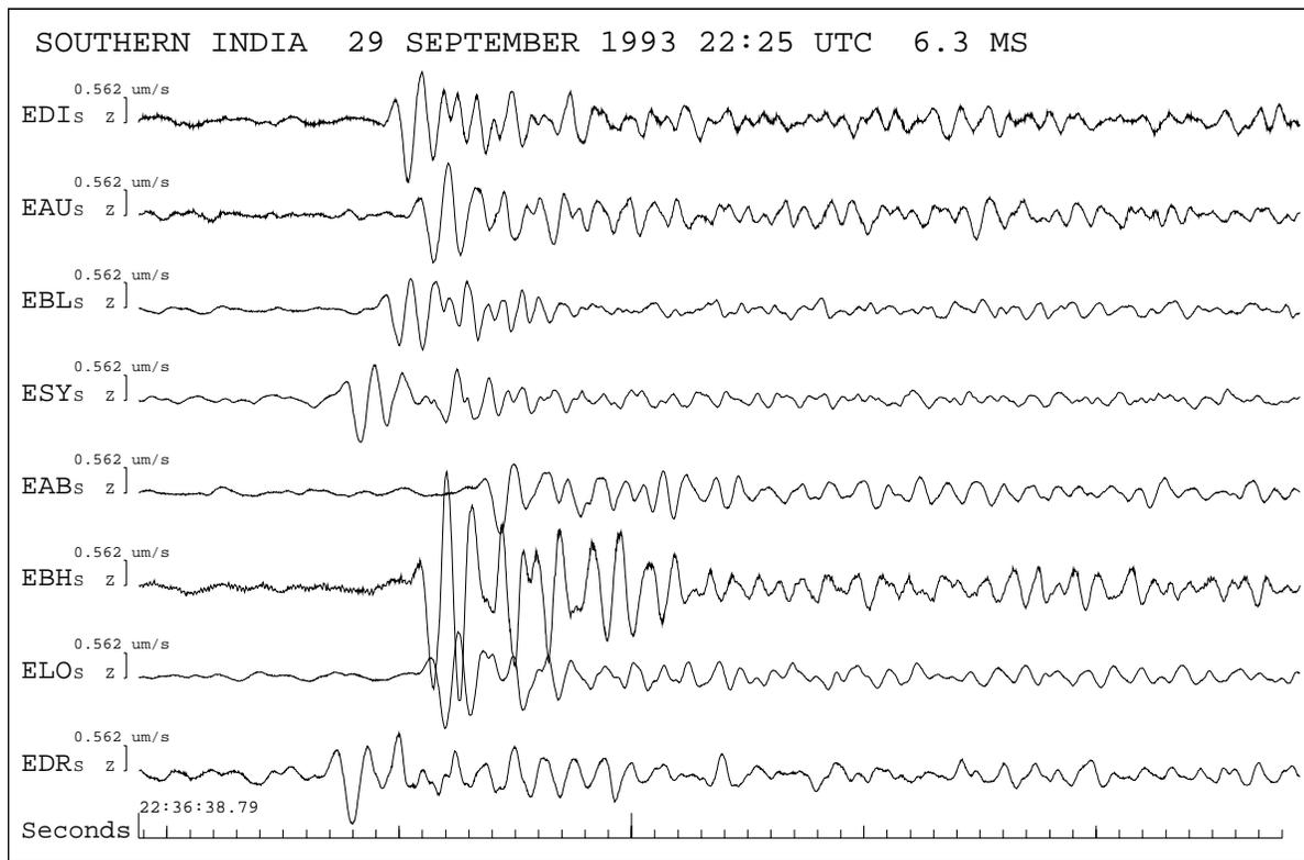
**Figure 15.** Seismograms recorded on the Lowlands network around Edinburgh from the magnitude 6.3 MS earthquake in southern India on 29 September 1993. Three letter codes refer to stations in Annex E.
