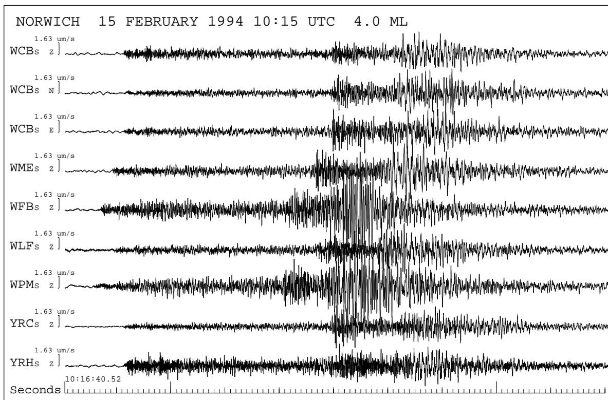
**Figure 10.** Seismograms recorded on the North Wales network from a magnitude 4.0 ML earthquake felt in the East Anglia region on 15 February 1994. Three letter codes refer to stations in Annex E.
