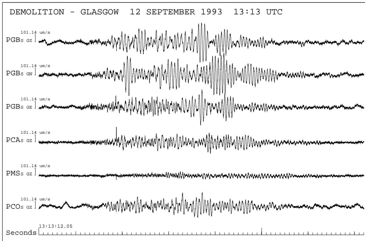
**Figure 13.** Seismograms recorded on the Paisley network from the Glasgow flat demolition on 12 September 1993. Three letter codes refer to stations in Annex E.
