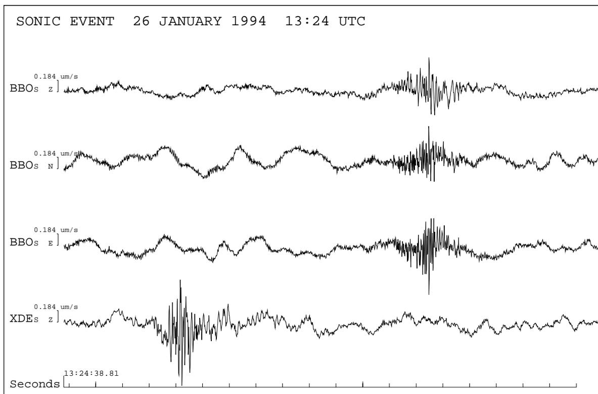
**Figure 12.** Seismograms recorded on the Cumbria network from a sonic event felt in the Workington area, Cumbria, on 26 January 1994. Three letter codes refer to stations in Annex E.
