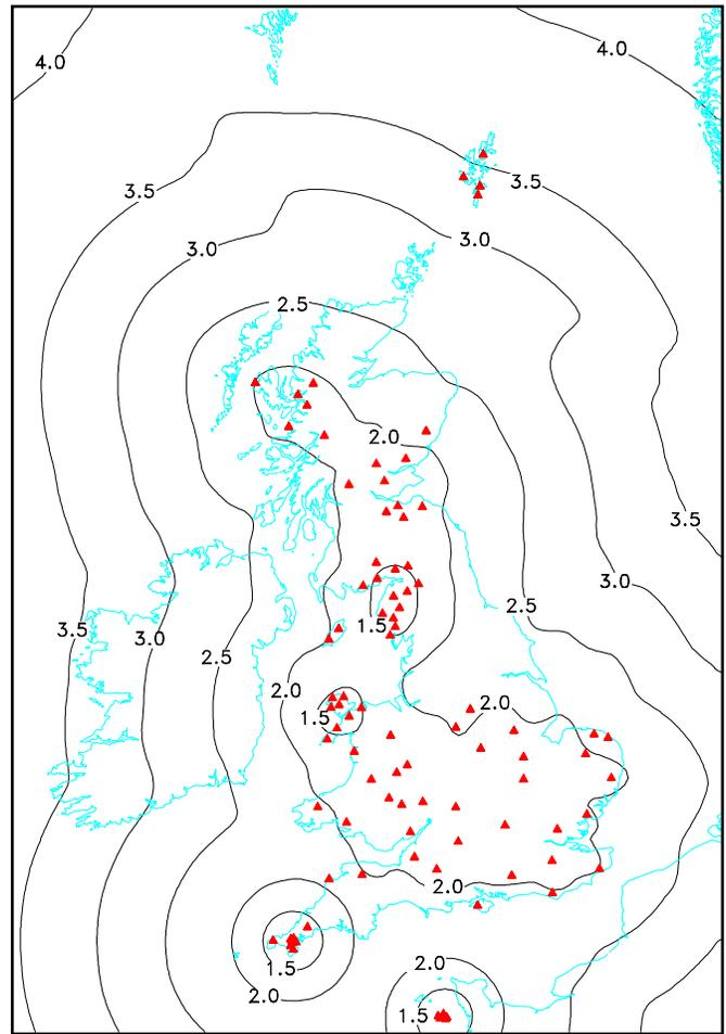
**Figure 6. Detection capability of the rapid access networks. Contours show the magnitude (ML) of an earthquake which would be detected by 5 stations in the presence of 20 nanometres of background noise at 10 Hz.**
