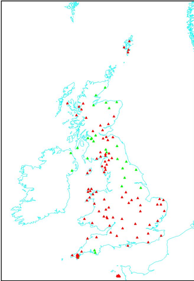
Figure 1. BGS seismograph network operational in March 1994. Colour coding shows the standard stations (green) and those upgraded to rapid access (red).
