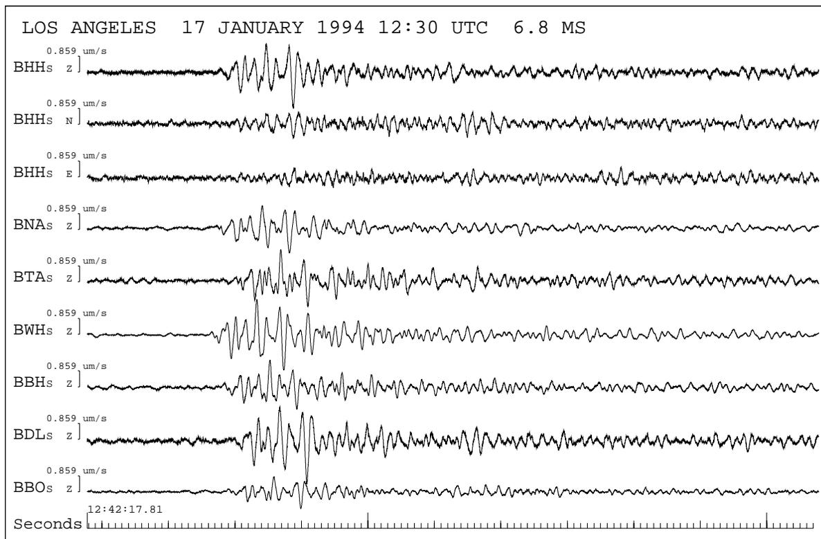
**Figure 16.** Seismograms recorded on the Borders network from the magnitude 6.8 MS earthquake in Los Angeles on 17 January 1994. Three letter codes refer to stations in Annex E.
