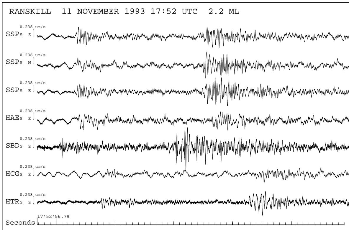
**Figure 11.** Seismograms recorded on the Hereford network from a magnitude 2.2 ML coalfield event felt in the village of Ranskill, Nottinghamshire on 11 November 1993 . Three letter codes refer to stations in Annex E.
