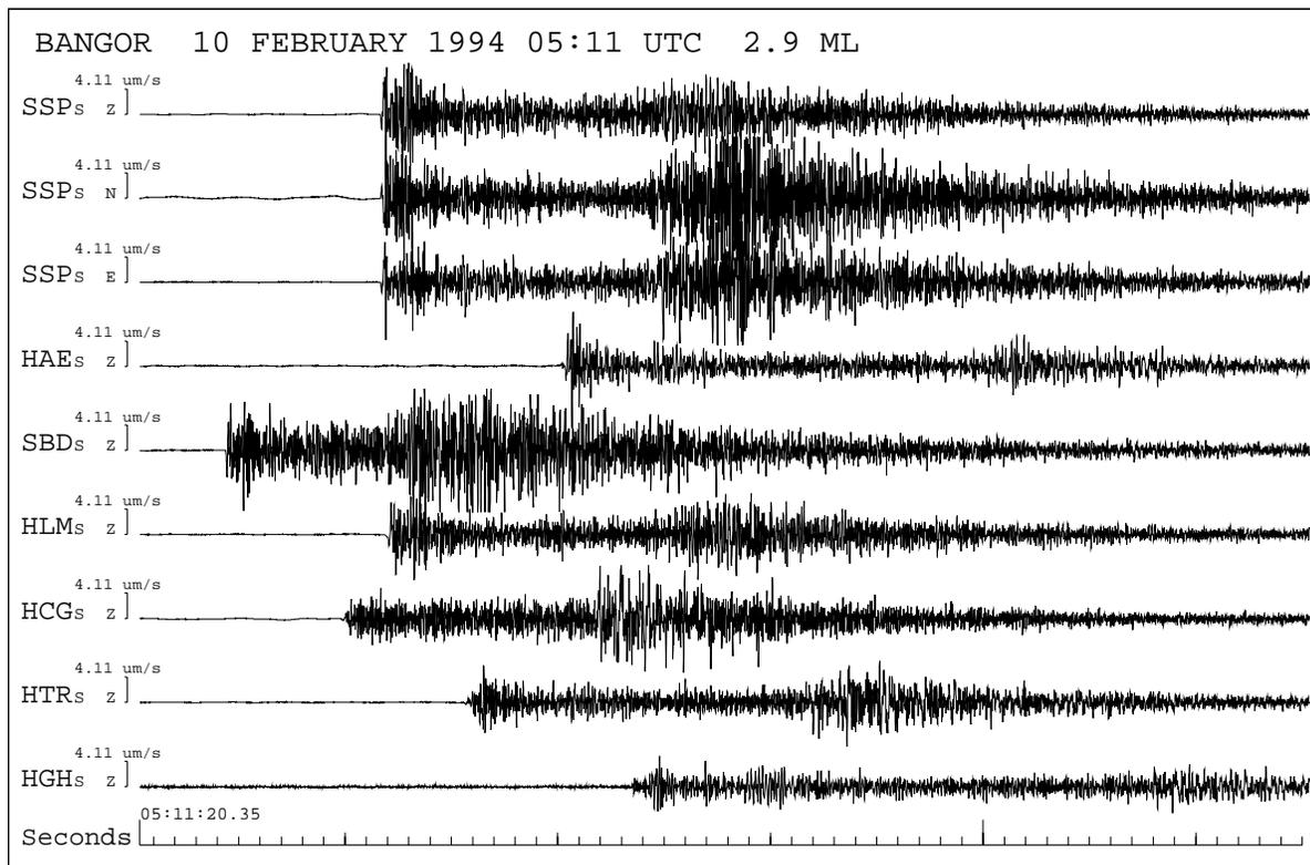
**Figure 9.** Seismograms recorded on the Hereford network from a magnitude 2.9 ML earthquake felt in the Bangor region of North Wales on 10 February 1994. Three letter codes refer to stations in Annex E.
